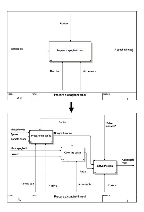
Figure 2. An illustration of the organisation of IDEF0 models. All models start with a context diagram, containing only one activity, which then is split into sub-activities, which in turn can be split into sub-activities etc.
